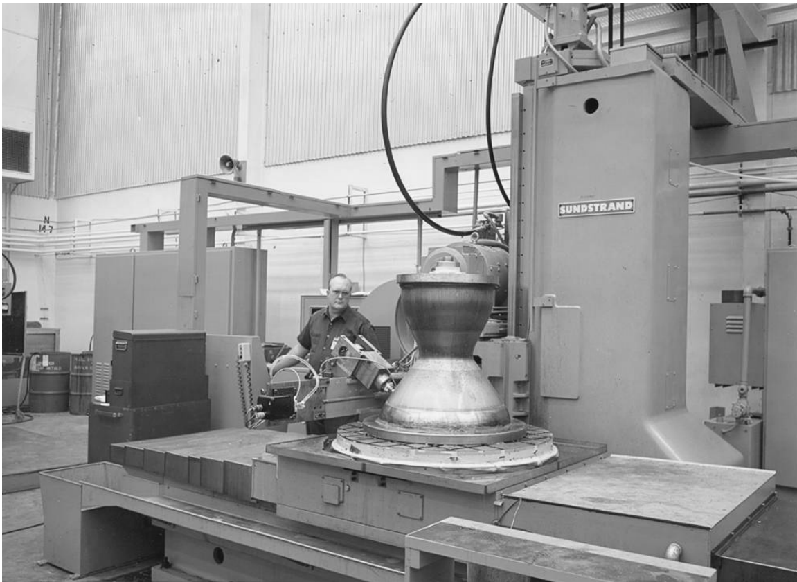
Figure C-28. Milling of the 390 Inlet Slots around the outer periphery of the Main Combustion Chamber of the SSME, on a Sundstrand Numerical Controlled Mill. Source: History of the Air Force Plant Representative Office Rockwell International Corporation Rocketdyne Division 1 January – 30 June 1974.
